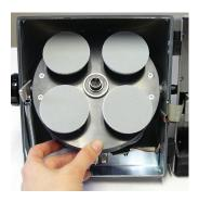
For discs that require heavy sanding you will need to flip the sanding head to the grey sanding pad side.
