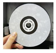
After every cycle your sanding pads will need to be cleaned, using the White Velcro side of your Cleaner Disc. Place Cleaner Disc in the unit with the Velcro side facing operator. Liberally apply WorkMate conditioning solution on Velcro. Cleaner Disc should appear to be soaked. Also dab solution on sanding pads. Close the door. Verify
