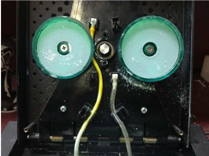
12. Re-Install the green lid screen, six screws, buffing pads, and center hub. The Hybrid is ready for use.
