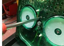
3. **Unfasten the compound tubing**. The line of tubing on the left is the compound tubing. To unfasten the tubing, pull the white nozzle out of the holder. (You may use pliers if needed.) Pull the tubing out from behind the pad satellite, and pull the tubing out of the bottom bracket.
