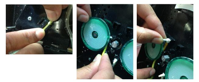
11. **Double check the installation of the lines.** Make sure the placement of the compound line matches the photo below.
