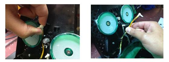
4. **Cut the nozzle from the tubing.** Position the scissors on the tubing so that you may cut right after the visible end of the nozzle. With the nozzle cut free, pry the remaining piece of tubing off the nozzle (or cut it away with scissors.)
