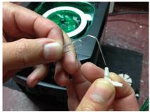
8. Reconnect the nozzle to the compound tubing securely.
