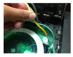
7. **Clean the nozzle.** Remove the nozzle from the hot water. Use a paperclip or a pin to clean out both ends of the nozzle.
