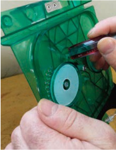
13. Using a firm blunt object, push the two fittings through the head assembly to completely free the tubing.
