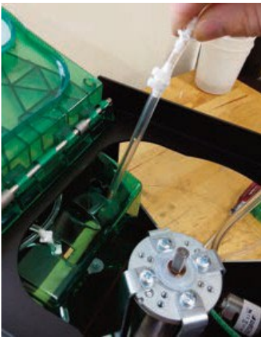
15. Replace with new tubing. Compound tubing is installed on the right side, water tubing on the left.
