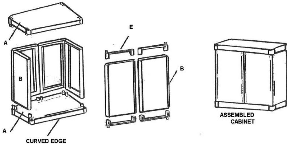
Step 2: Align the base and top marked A with the curved edge facing towards the front as shown above and press panels (B) over the posts so they fit in.
