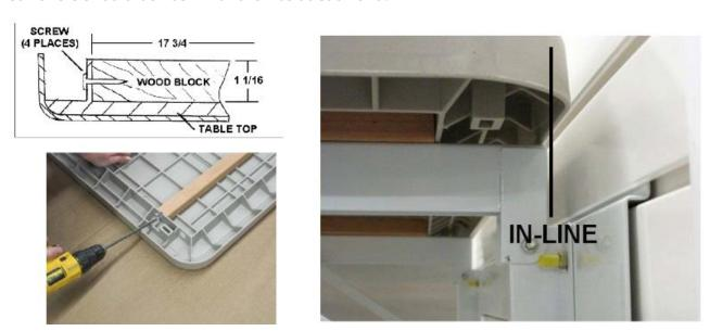
Step 6: Place the table top back edge in line with the folding bracket assembly.
