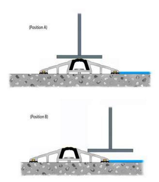
(Position A) The Threshold Seal may be fitted to the floor directly beneath the door so that the door closes on the top of the Threshold Seal.
