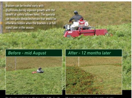
Glyphosate applied at a dilution rate of 20:1 with a work rate of up to 7 acres (2.8Ha) per hour using this 2.5 metre wide model. Work rate dependent on forward speed, terrain and ground conditions.
