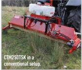
facing front or rear depending on the required fitment to a tractor. A complete 12v wiring harness and control box is supplied on all models together with a chemical supply system - various tank sizes are available as well as an optional bout marker see page 2 for further details.
