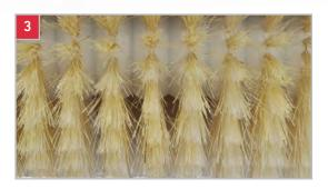
The unique nature of this Logic patented brush (left) is fundamental to the success of the system. It is a mixture of absorbent natural fibres and synthetic fibres in interlocking rings of bristles mounted on a central shaft with a slight gap between each of them to allow plants to 'comb' through, delivering a high dose of chemical in one pass.
