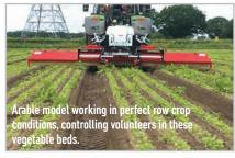
These arable examples of weed wiping (above) show very clearly how accurate the system can be to control targeted weeds growing above the host crop. This contained system is accurate and safe allowing operation close to watercourses and buffer zones. Wiping can be carried out in windy or changeable weather conditions which increases the opportunity for weed control considerably.
