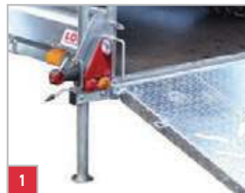
1 Prop stands to support the trailer when loading vehicles.
