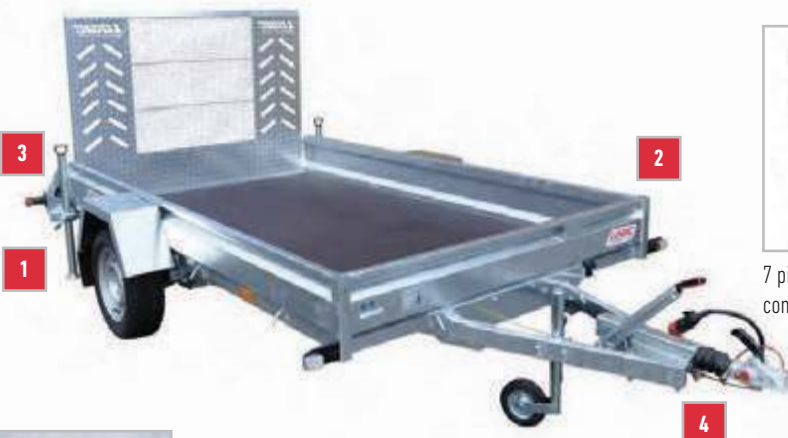
2 Monoque construction with 'A' frame drawbar, Al-Ko suspension, one piece axle (1300kg) featuring rubber progressive action with excellent dampening. All protected with hot dipped galvanising for long life.
