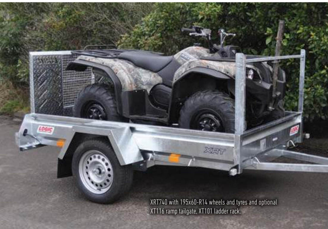
Optional XT116 metal loading ramp/tailgate, for loading ATVs, garden machinery, etc.
