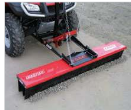
S221 snow plough 1.4 metres wide. Sturdy construction with heavy duty blade, rubber wearing strip and manual raise and lower.
