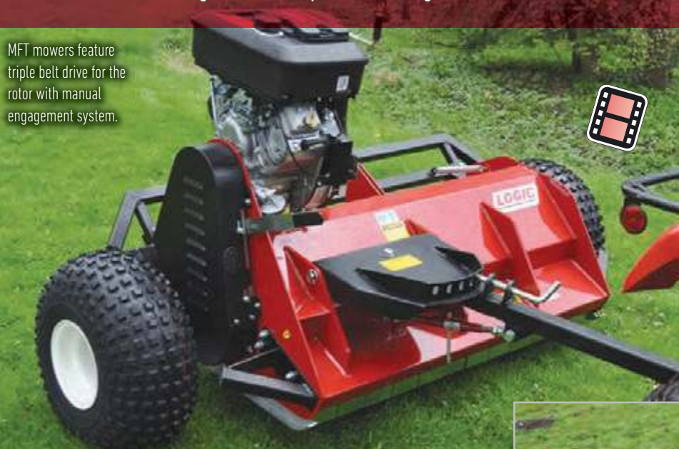
MFT120B18FW 'Scrub Buster' model fitted with optional flotation wheels.
