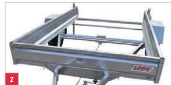
2 Monoque construction with 'A' frame drawbar, Al-Ko suspension, one piece axle (1300kg) featuring rubber progressive action with excellent dampening. All protected with hot dipped galvanising for long life.
