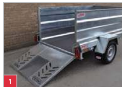
Optional XT116 metal loading ramp/tailgate, for loading ATVs, garden machinery, etc.
