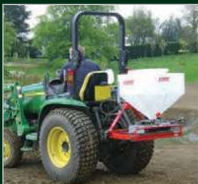
TPL115 Mounting frame (left) for 3 point linkage on tractors, suitable for larger electro broadcasters when spreading grass seed mixtures, fertilisers, etc.
