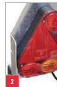
Protected light cluster with inbuilt triangle and lenses.
