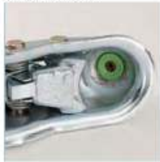
Blocked ball socket
