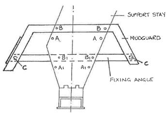
Position the mudguard fixing angle behind the support stay and line up the corresponding holes with the mudguard.
