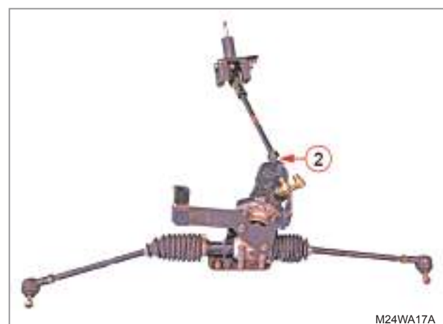
11. Unscrew the steering gearbox bracket mounting bolt (1) to remove the gearbox assembly (2).
