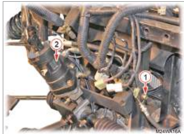
10. Unscrew the mounting nuts (1) of the tie rod ends (LH, RH) to remove the tie rod (2).
