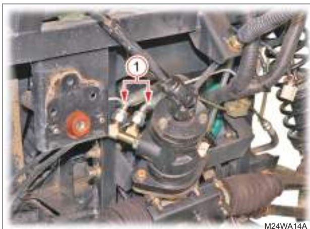
9. Disconnect the torque generator hydraulic hose (1).
