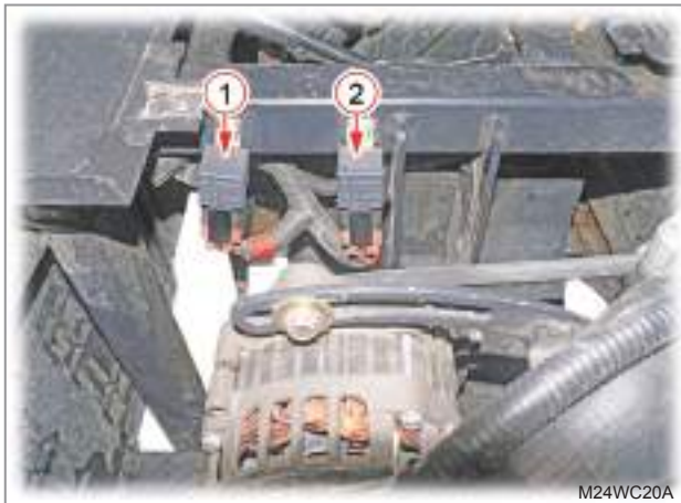
(1) Power relay (2) Glow relay
