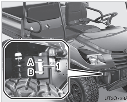
(1) Auxiliary coolant tank (A) MAX Limit (B) MIN Limit
