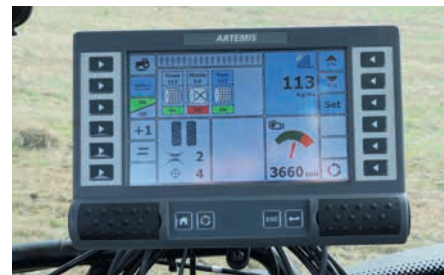
An RDS Artemis controller monitors tank fill level, seeding rate, fan speed and coulter; precision farming software can be unlocked to offer variable rate and recording functions; the drill is also ISO-compatible.
