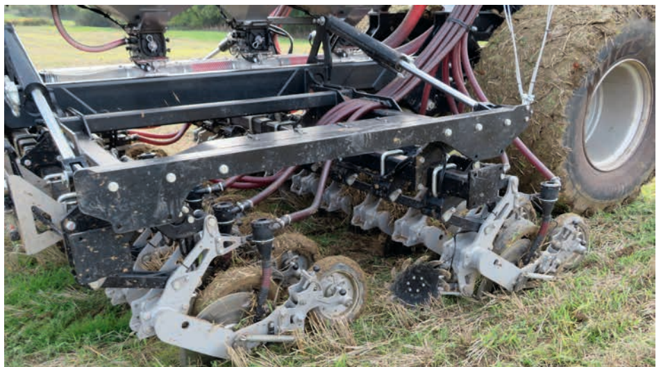
The disc unit is angled at 20° to the vertical and slightly to the horizontal to create a slice similar to a plough mouldboard.
