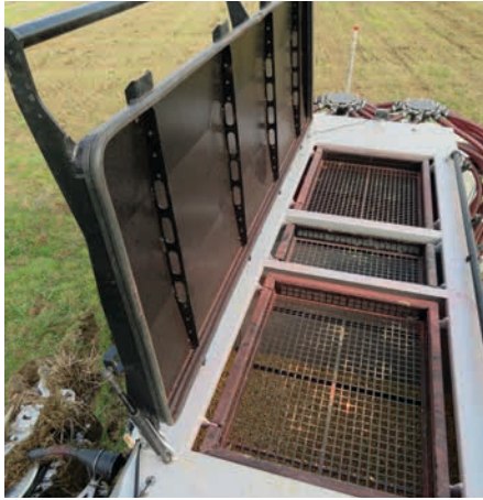
The main tank is specified with two hoppers as standard, with the option of three, its 4,400 litres being split 60:40 or 40:40:20.
