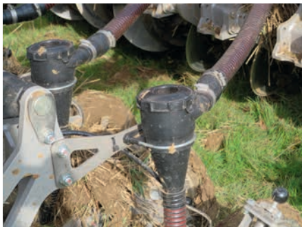
Diffuser units between the distribution heads and the coulters combine air and seed in an anti-cyclone which forces the air out of the top while seed drops down to the seeding boot via gravity. In the event of a blockage, seed comes out of the top, and is visible from the cab.
