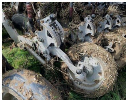
Pressure on the disc is repeated on the rear press wheel, helping to fully close the slot.
