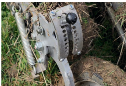
Individual depth control for each row unit allows seed to be planted at different depths when establishing companion crops or different cover crop seeds.
