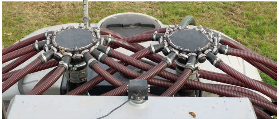
The two distributor heads are plumbed front to rear so you can divert the flow from either the front or rear metering units, for example to send oilseed rape from the to the front coulters and buckwheat to the rear and slug pellets to both.
