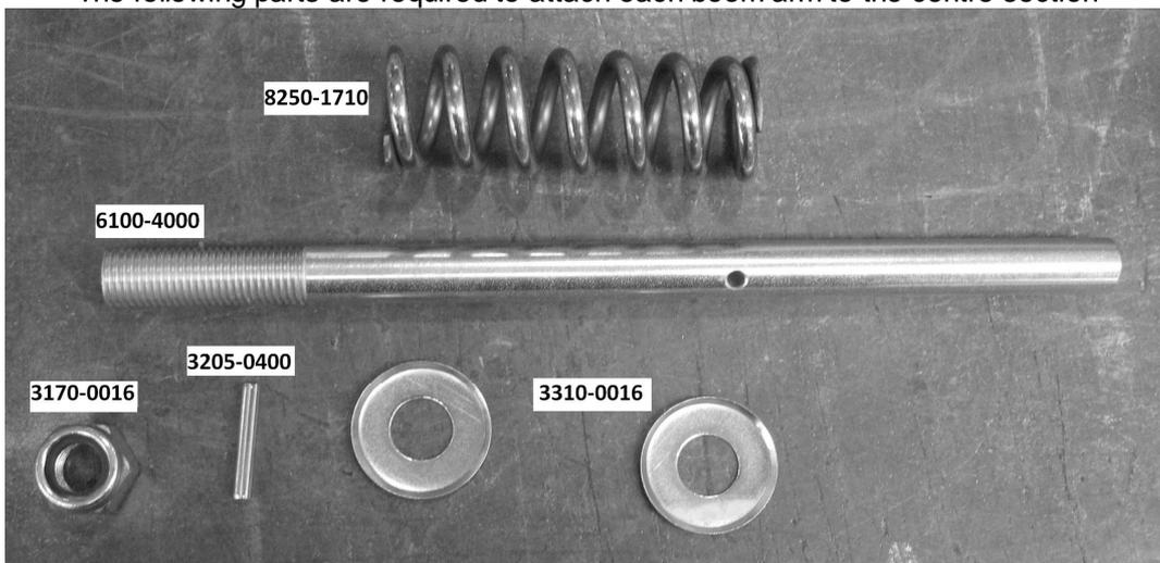
Assemble the pivot as shown below. **Apply grease between the cup and round tube to ensure smooth operation.** Use a pair of pliers to hold the roll pin when doing up the nyloc nut with a spanner.
