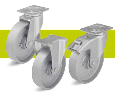
Wheels: G series - Made of grey cast iron, with grease nipple, lacquered, silver. Bearing types: Plain bore or two pressed-in ball bearings. Detailed description: Page 320 and 50
