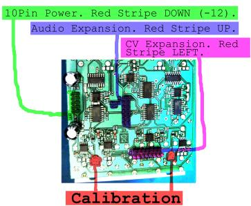
Calibrating the uHC should not be necessary, but the 1V/Octave scale can be calibrated by turning the trim pots behind each channel. Use bandpass output and sine-wave input. Match the frequency at CO to get resonance boost, and check at C5. Adjust the freq knob to check resonance boost. If the boost is at higher frequency than played, turn the trimmer clockwise.
