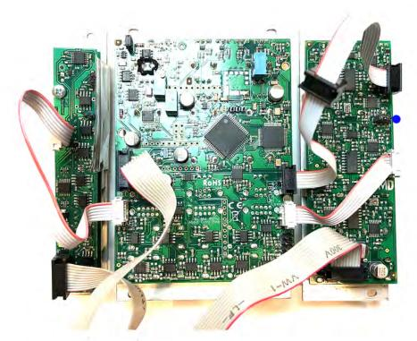
Three connector cable in use on PDO MKII. Middle header is left unused.
