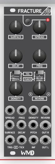
TRIG-{ ACC }-TICK: Trigger, Accent, Tick. Sending a trigger into TRIG starts a particle burst. A louder, longer, accented particle burst is played if tick is high when the TRIG event occurs. Send a trigger into TICK to play a single particle sample on the rising edge.
