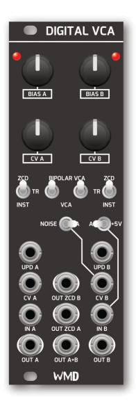
OUT A+B: This output mixes the A and B outputs at unity gain.
