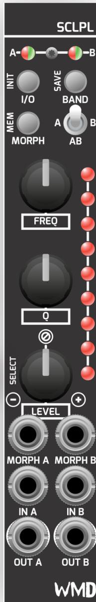
Channel LED Display: Indicates selected band and bypass status.
