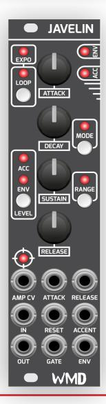
ACCENT (CV): Putting a positive signal into this jack creates an accent by allowing the envelope to attack to a higher voltage. A higher voltage at this CV will correspond to a more dramatic effect. Use a sequencer to jump between different accent amounts for even more dynamics. Holding MODE and pressing LEVEL will toggle "accent stacking." This feature slews the accent response while it's enabled. The ACC LEVEL LED will blink 3 times when this feature is enabled. Once when disabled.
