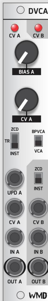
**CV B LED:** Displays the current attenuation ratio of IN B to OUT B.
