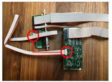
To connect Performance Mixer and PM Channels, repeat the two steps above, connecting the PM to the DB25 expander.
