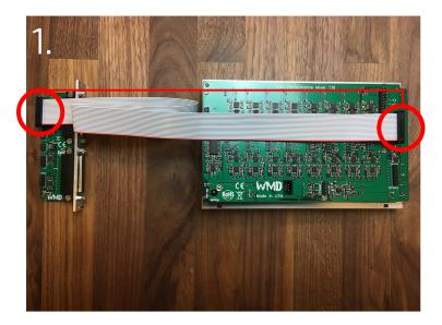
First, connect the far-right 20 pin connector on the Performance Mixer to the 20 pin header on the very top of the DB25 expander with the included 20 pin ribbon cable.
