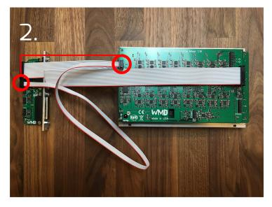
Next, connect the top-most, far-left 6 pin header on the PM to the 6 pin header on the DB25 expander directly below with the included 6 pin ribbon cable.
