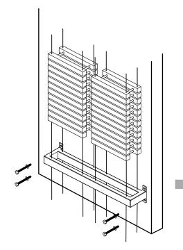
Before you pull down your installer can draw a level line on the wall to ensure that the wall mount screwed into the wall leveled. Use the appropriate screws, bolts and washers (4 sets) to secure bottom bracket to wall.
