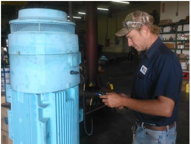
EXPERIENCED field service engineers and technicians are available to test new and existing pumps. We test the hydraulic conditions (flow rate, pressure and temperature), the mechanical conditions, level, and the vibration trending, vibration measurement and trim balancing using a Vibscanner.
