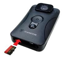
1. Insert a microSD memory card into the card slot on the bottom of the camera.
