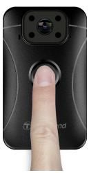
At night or in low light conditions, the Infrared LED mode will be activated automatically; the four Infrared LEDs will then light up. Please keep the DrivePro Body 10 at least 50 centimeters away from the object to avoid misjudgement of the light condition due to a reflection of LED light.
