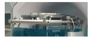
Stealth reference chamber including special holder for Varian<sup>®</sup> Halcyon™ / Ethos™ (\*) – Linac allows field-size measurements up to max. 28x28 cm without excursions into Linac room for reference chamber re-alignment.
