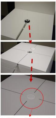
An RW3 cap to fill out the gap in the  $\,$ plate lid is included in the chamber package.
