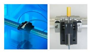
The horizontal orientation is shown with the mounting of the CC13 Ion-Chamber. The vertical orientation is demonstrated with the mounting of the RAZOR™ Diode.
