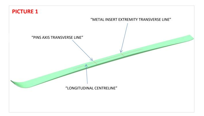
A) **BOOT CENTER METHOD**: locate the boot center mark indicated on the skis; place the boot on the ski with its tip facing the tip of the ski; match the boot center indicator marked on the sole with the boot center mark indicated on the ski; keeping the boot in the desired position and aligned with the longitudinal centerline of the ski, mark the "**PINS AXIS TRANSVERSE LINE** " matching to the front metal insert on the boot .
