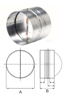
Backdraft dampers are designed with galvanized steel collars and have lightweight aluminum damper blades. They are spring loaded for positive closure.
