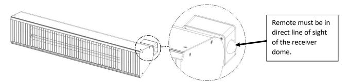
In remote mode the heater has the option to run at 50% or 100% power. Each emitter is controlled separately using the up and down arrows on the remote. Pressing the up button (^) will turn the upper emitter on. Pressing up again will turn the upper emitter off. Pressing the down button (^) will turn the lower emitter on. Pressing down again will turn the lower emitter off. Pressing the (all) button will turn both emitters on, pressing it again will turn both emitters off.
