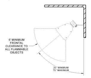
The angles of attachment are 20° to 70°, measured from the mounting wall.
