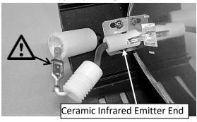
7. Bend the metal tabs to remove the small reflector shield sheet metal parts. Hold on to these pieces. This will allow you to slide the emitter into a bigger cavity to remove it from the reflector and heater body. Properly dispose of the broken emitter at your local recycling center.
