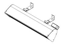
short part of the bracket. Brackets should be attached as shown below. **NOTE:** Wall bolts or anchors are not supplied. Select an appropriate size to provide adequate support for the weight of the unit and taking into consideration any wind load conditions.
