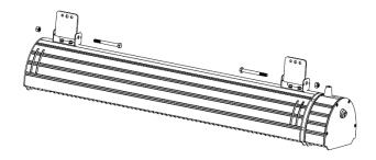
4. Select the installation location on the wall by identifying the studs or structural beams that will allow the heater to be securely attached.
