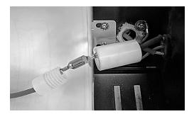
11. Carefully replace the protective aluminum grille and screw the protective end cap in place.
