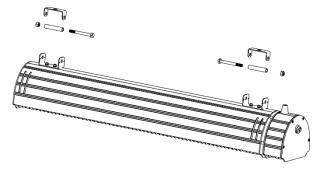
3. Install the two wall mount pivot brackets using the screws removed in the previous step.
