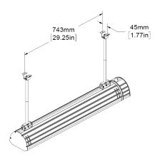
5. The heater can be hung vertically or pointed at a maximum angle of 45° from vertical.
