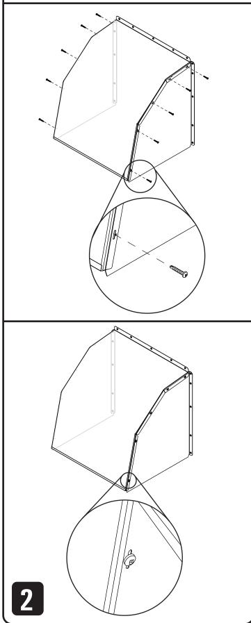
If mounting weather hood over a shutter or other inlet, ensure that hood placement will not block shutter movement.
