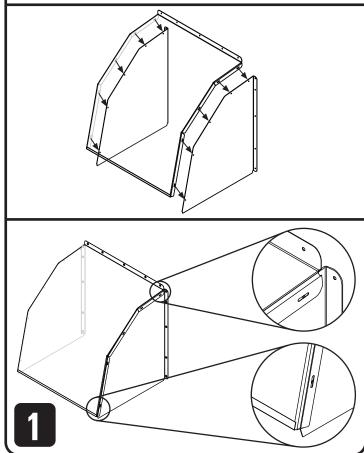
To secure assembled unit, join the edges and tabs together using the included #10 x 1" Square Head Tek Screws as shown below. (On sizes 12".30" use 5 screws for each side, on 36" use 10 screws per side, and on 48".50" use 11 screws per side.)
