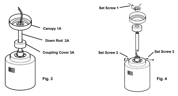
• Run the black and white wires and safety cable through the center of the downrod (2a). Use the gold keeper pin (Photo 7) to connect the motor to the downrod. Ensure the three set screws, shown above, are installed and tight. These screws prevent the torque of the motor from rotating the fan housing and causing a knocking sound during the fan startup process. If you fail to tighten these screws the fan will seem to be out of balance. These screws MUST BE TIGHT.
