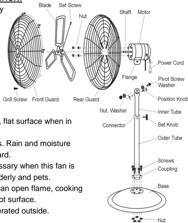
**WARNING:** be sure front and rear guard screws are completely screwed down in locking position before operation.
