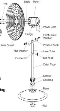
11. Comp lately tighten grill screws washers on front guard and into back guard.
