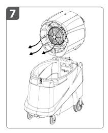
Once installed, the **atomizer** (metal disk) will be facing the **water tank**, air will be blown *over* the **water tank** when the Power Breezer is turned on.
