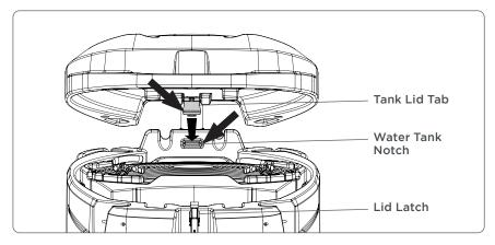
Note the lid tab on the back underside of the lid.
