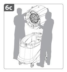
6c. Once again, lift the fan head and align it with the fan head support pole. Once the fan head is seated on the support pole, rotate the fan head horizontally until you feel it engage with the support pole.
