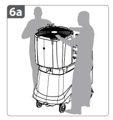
6a. Lift the fan head straight up and out of the water tank. Carefully rest it on the edge of the water tank.
