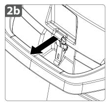
**2b.** Finish opening the **lid latch** by pulling the upper portion of the latch forward and away from the lid.
