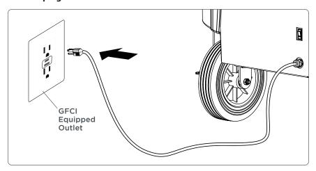
**NOTE:** A live power outlet can be verified when the Power Breezer is **plugged in and powered off** by pressing the **oscillation** or **atomizer buttons.** The LED lights will dimly illuminate when either of these buttons are depressed.
