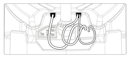
**4a.** Route the **fan head power cord**, **atomizer drain hose**, **and water inlet hose** through the openings in the back of the **water tank** as shown above.
