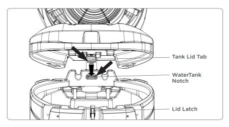
Note the tank lid tab on the back underside of the tank lid.
