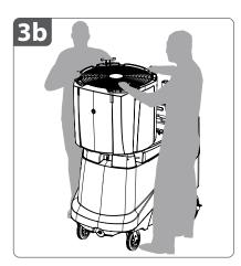
**3b.** Carefully rest the **fan head** on the **edge of the tank**.
