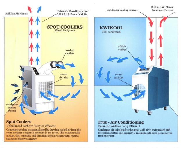
Commercial & Industrial Use • Air / Water-Cooled Units • Split Configuration Available • Manufactured in USA • Distributorships Available
