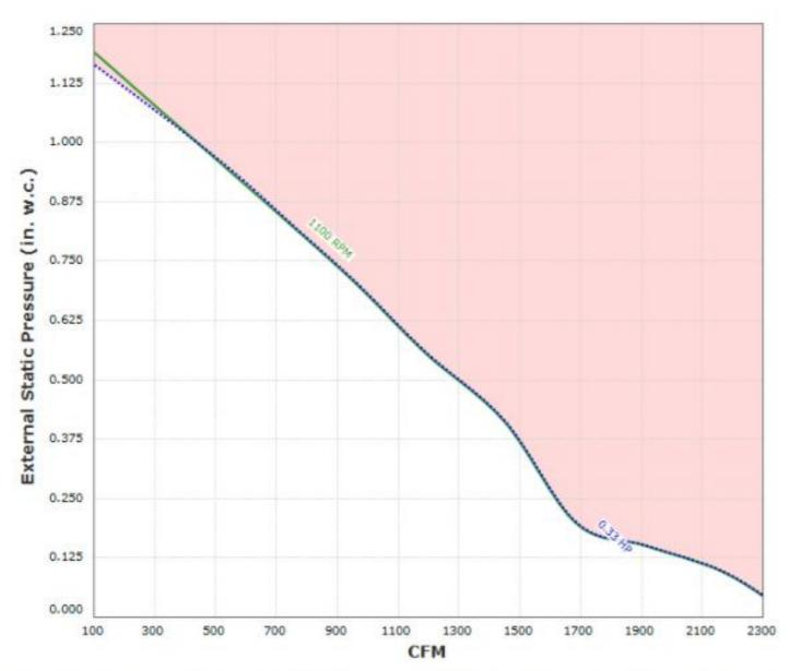
Performance shown is certified for Installation Type A: Free inlet, Free outlet. Performance ratings do not include the effects of appurtenances in the airstream. Power rating (BHP) does not include transmission losses.
