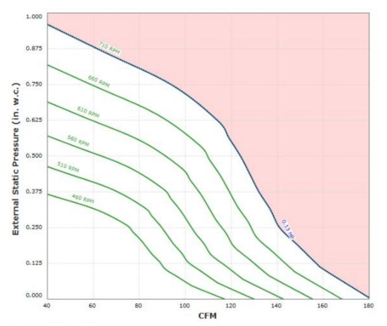
Max Sizeable RPM = 710 RPM. Curve shown extended beyond this point for reference only. Motor Broan 100 W, 120V has an rpm range of 426 to 710.
