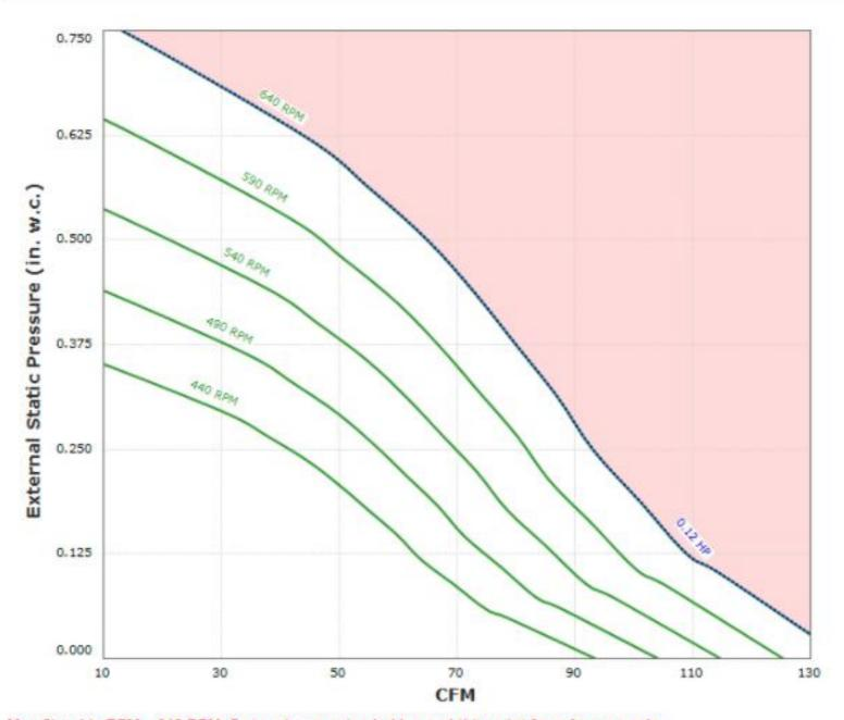
Max Sizeable RPM = 640 RPM. Curve shown extended beyond this point for reference only. Motor Broan 87 W, 120V has an rpm range of 400 to 640.
