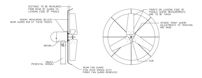
IMPORTANT NOTE: THE LEADING EDGE OF THE FAN BLADE PADDLE IS THE EDGE OF THE PADDLE WHICH LEANS CLOSEST TO THE REAR GUARD - THE LEFT EDGE OF THE FAN BLADE PADDLE AS LOOKING AT THE BLADE THROUGH THE REAR GUARD.
