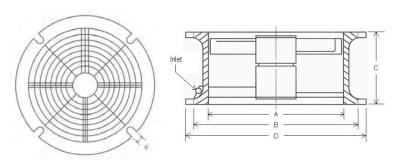
A – Internal Diameter B – Bolt Circle C – Height D – Outer Diameter E – Butterworth (Flange)
