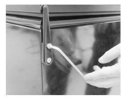
3. Loosen the upper hinge and remove it (4 mm Allen key).
