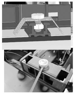
10. Unscrew the lock pin (using the flat-headed screwdriver) and remove it.
