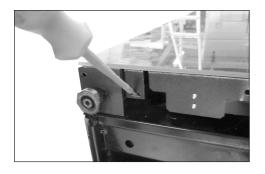
4. Dismount the bottom cover (the built-in snap function in each side can be unsnapped with the flat-headed screw-driver).
