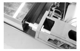
26.Push the door back in place over the hinge pin and pull the wires simultaneously so the wires do not get stuck.
