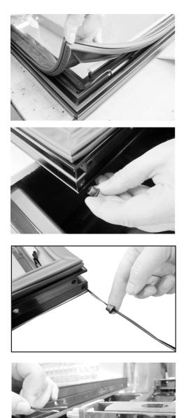
19. Make sure the wires are fitted into the plastic groove and mount the gasket. It's important to check that the sealing strip provides a tight seal all the way round.
