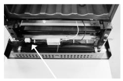
5. Place the bottom cover with glass front down, on an additional support, so the wires are not stretched.
