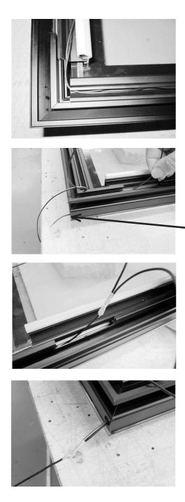
16. Replace the wires into the plastic groove and lead them to the other side.
