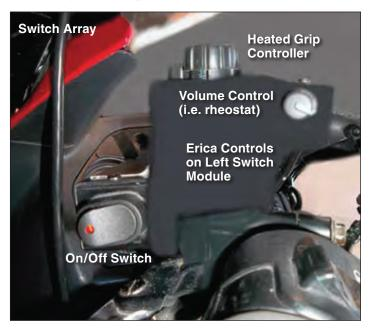
Clearwater has many ready-made attachment mounts for most motorcycles. There were no mounts for my motorcycle so I made my own mounts and enclosures to place the controls on the left handle bar switch array. My motorcycle has only one reinforced attachment point available but the mount design worked well.
