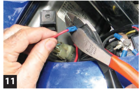
11 Because LEDs draw so little power (only 12 watts for the Glenda at full power), we used small crimp connectors for some connections. Use the correct tool when crimping the wires; don't use pliers as the wires can come loose.
