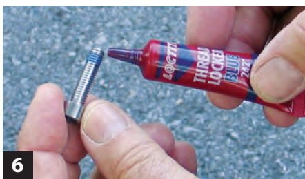
6 Motorcycle engines vibrate, so we're using Thread Locker from Loctite to keep the bolts from backing out.
