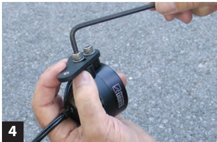
4 The brackets are fastened to the lights prior to mounting them on the side of the fender. We hand-tighten the fasteners as the lights will have to be adjusted once the bracket is mounted on the bike.
