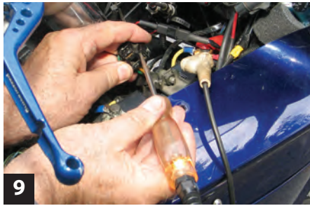
9 Use a 12-volt test light to locate a switched power source and the wire that operates the high-beam circuit. These will be connected to the dimmer and relay that comes with the wiring kit.
