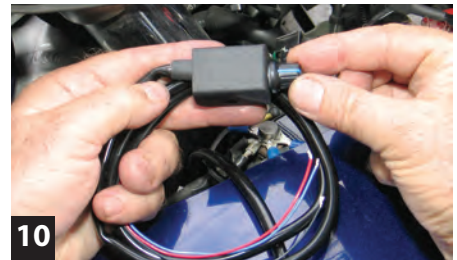
10 The Glenda lights use a rotary dimmer to adjust the level of light intensity. Light output can be modified to suit riding conditions and to keep from blinding oncoming drivers.
