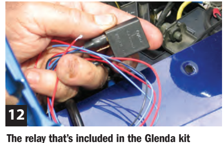
12 The relay that's included in the Glenda kit switches the lights to full power automatically when the high beam is switched on. Use of the relay allows the lights to be dimmed for normal riding and switched to full power when you really need to get noticed.
