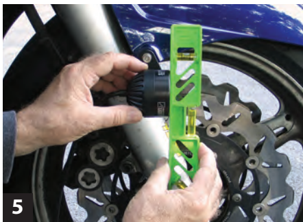
5 With a rider holding the bike upright on a level surface, the lights are aimed using a level. The housing should be 90 degrees to the ground. A 2' x 2' board can be substituted for the level.
