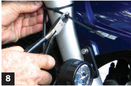
8 Tie wraps are used to affix the light's wires. When routing the wiring, make sure to leave enough slack for suspension movement. Brake lines are good for attaching wires to the bike.
