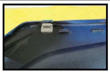
Carefully align the new tab to the center of the masking tape location. Press new tab in place. Hold in place with medium pressure for 10 seconds. The adhesive tape we use is very strong and the bond increases in strength after about 24 hours. It is the same tape that auto manufacturers use to attach model badges on trunk lids. If applied correctly, it will last a very long time.
