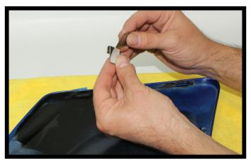
Using a sharp edge, peel off the adhesive covering on the back of the tab. Use a hair dryer to warm up the adhesive and the fairing where the tab will attach.
