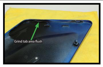
Remove panel and set shiny side down, on a table protected by a towel or other soft cloth. Carefully grind off the remaining plastic tab to reveal a smooth surface that resembles the part of the panel without the tab. Clean this channel out to allow the new part to fit flush.
