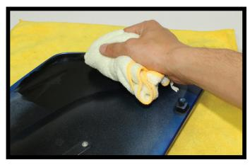
Remove the fairing and use denatured alcohol to clean the surface where the new tab will attach.
