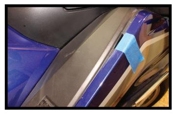
Fit fairing to bike and put a piece of masking tape on fairing, marking the spot where the old fairing tab lines up with the fairing tab hole on the bike.
