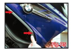
Once lower portion of the fairing is pulled out, slowly lift out top tabs. Make sure fairing doesn't snag on anything while lifting up. (If done incorrectly, the top tabs can easily break). [Fig. R6]
