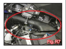
Removal of the air inlet tube can be made easier by first removing the (2) circled screws and pull out tab holding down the body panel marked in [Fig. R8]. The front portion of the lower body panel can then be pulled
