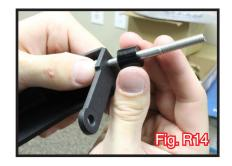
Attach both spacers to the two bracket holes seen in [Fig. R15].
