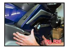
Reinstall torx bolts under fairing assembly. [Fig. R27]
