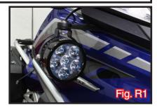
First, remove the two bolts under the fairing using a #25 torx wrench.
