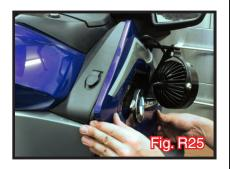
After top tabs are aligned, line-up and push in (2) lower tabs. The light bracket wil be fairly tight against the fairing.
