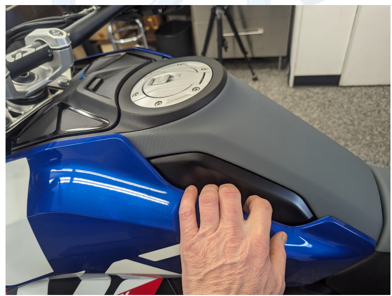
6. After the screws are removed, the panel can be pulled off with a firm pull
