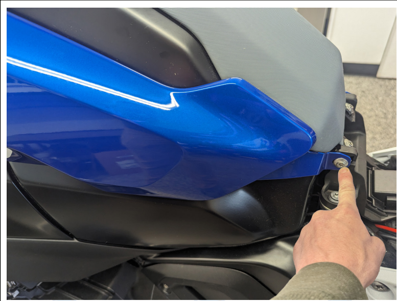
6. After the screws are removed, the panel can be pulled off with a firm pull
