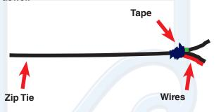
5. Route the wires along the frame as shown (this process can take some time as fishing the wire through can be difficult, you don't need to take off the fuel tank)
