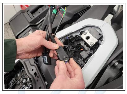
4.Plug in the canopener's connector into the port on the bike
