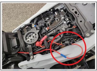
7. Attach the power wire to the positive and negative termal making sure to remove the negative first and then putting it back last
