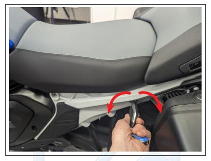
1. Remove the seats, ensuring to disconnect the seat warmer cables
