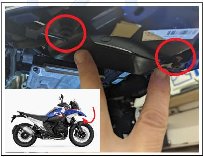
4. The nose piece can be removed with a firm pull from the top and the bottom pulling diagonally upwards. We also recommend digging into the fender from under the blinker as it helps to release a compression fitting
