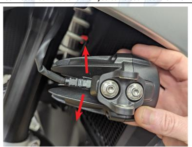
1. Take out these three screws on both sides of the bike. On each side, two are T25 and one is T40
