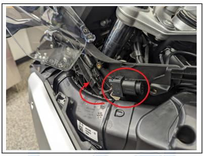
2. To do this, release the clip sliding the connector off towards the front. Flip the connector forward and zip tie it in place
