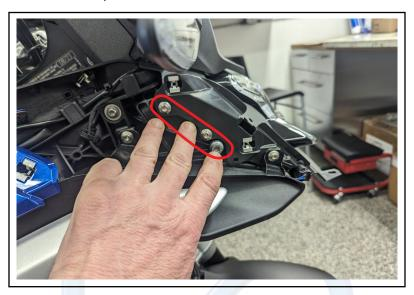
2. Install the left and right brackets by inserting them from the bottom of the bike. On each side, you will use two of the provided M5x20 screws (four total) in place of the T25 screws that were removed before. Additionally, you will reuse the T40 screw that was originally in place. Don't tighten all the way yet
