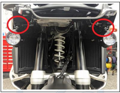
a. To do this, carefully pull the two clips holding the connector outwards and then you can disconnect the wire
