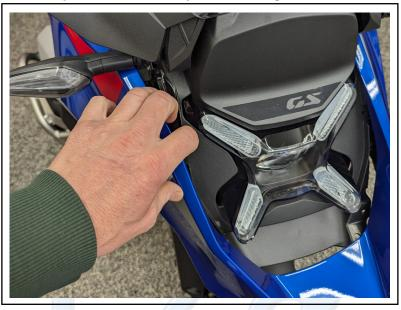
5. Take off the side panels using a T25, there are two screws
