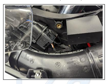
1. Before routing the wires remove these two panels
