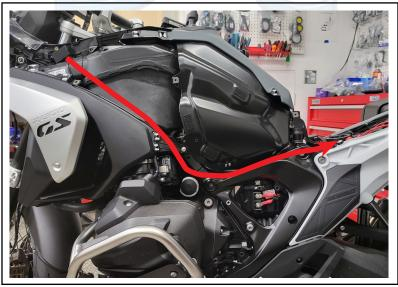
6. Attach the fuse to the red wire using the provided posilock
