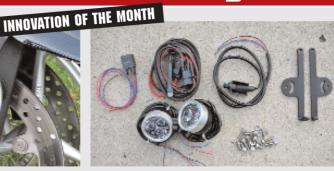
Lumen output at full power is advertised as 550, or approximately the same as a 50 Watt halogen bulb as commonly used on driving lights. However, the Glendas require only 12 watts each at full power, meaning that a pair of Glendas draws less than half the current of just one traditional driving light. For riders in need of additional lighting on bikes with limited alternator capacity, such efficient power consumption can be quite important.
